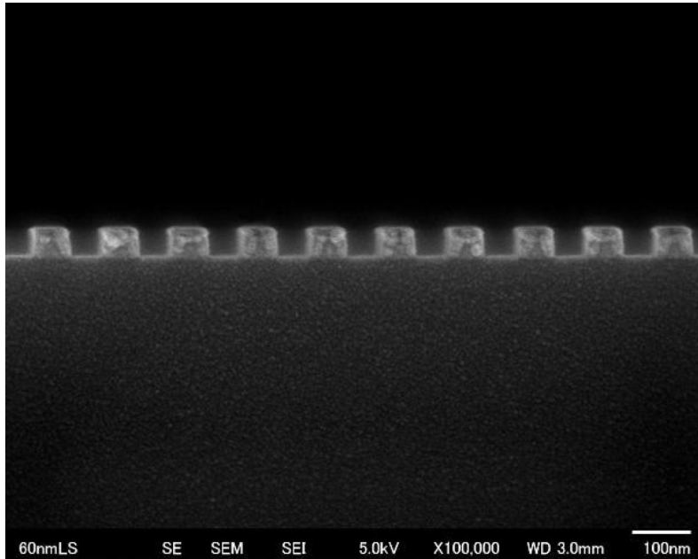
Cross sectional SEM image of 60nm L/S
